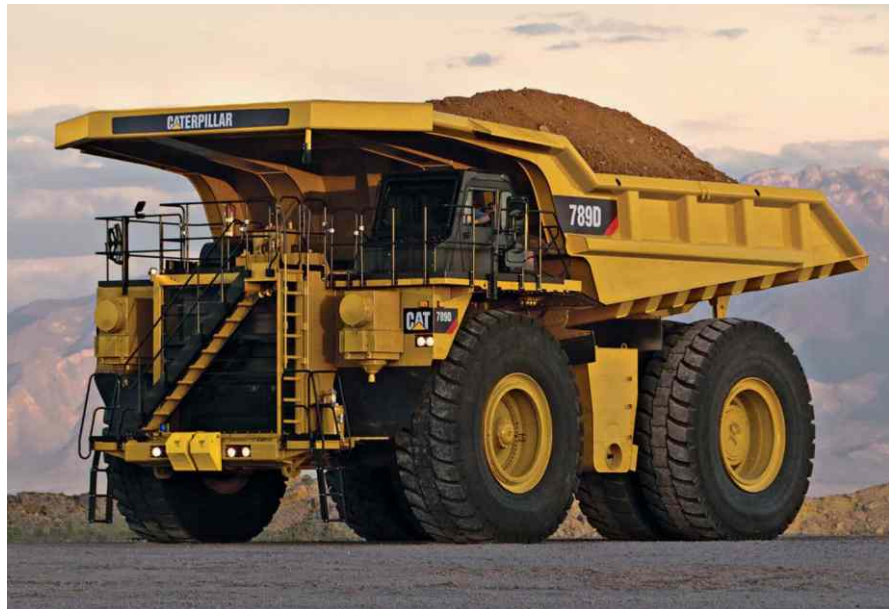
The latest generation CAT 789D has a nominal payload capacity of 200 tons (181 metric tonnes)
